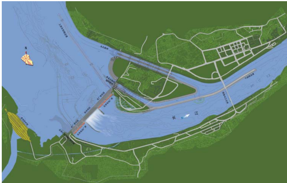
Key structures layout for Three Gorges Project
