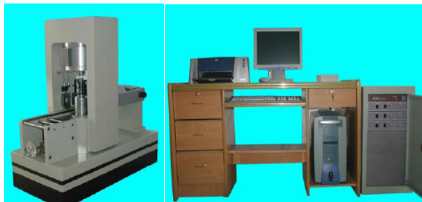
图1 RMT-150C型岩石力学试验系统及控制系统 Fig.1 Rock mechanics testing system RMT-150C and control system
