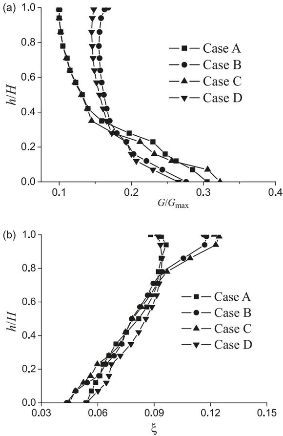
**Fig. 9.** Distributions of nonlinear soil properties at the downstream surface for the four cases A, B, C, and D referred to in Table 1: (a) normalized shear modulus, (b) material damping.
