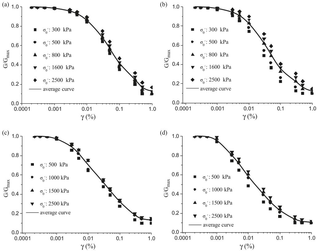
**Fig. 3.** Correlations between  $G/G_{max}$  and effective confining pressure for four types of soils: (a) core material, (b) filter material, (c) shell material, (d) transitional material.
